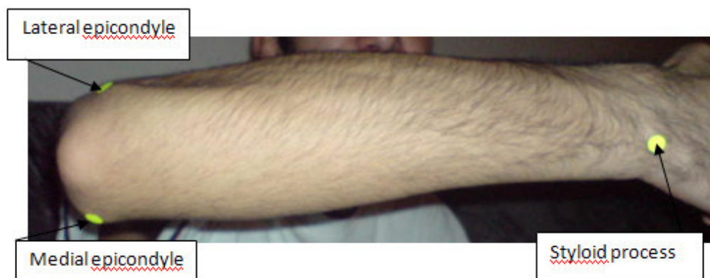
Figure 3-3: Markers on the arm (lateral epicondyle, styloid process and medial epicondyle which are used to study forearm movement).
