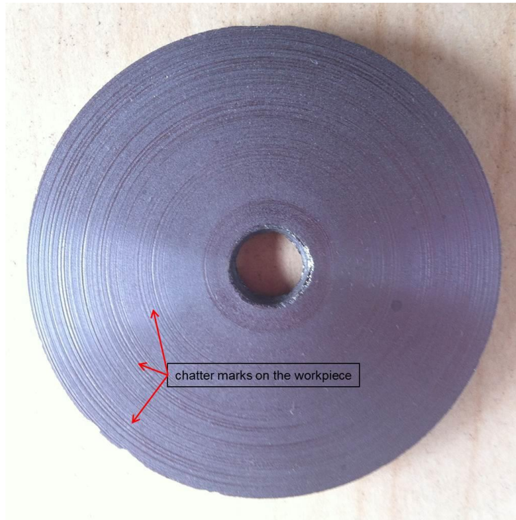
Figure 6.8 The chatter marks on the silicon workpiece taken after third cuts
