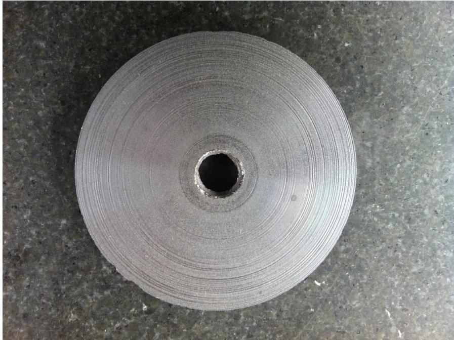
Figure 7.1 Poor quality of the machined surface from diamond cutting silicon wafer caused by rapidly worn tool, cutting heat and thermal effect
