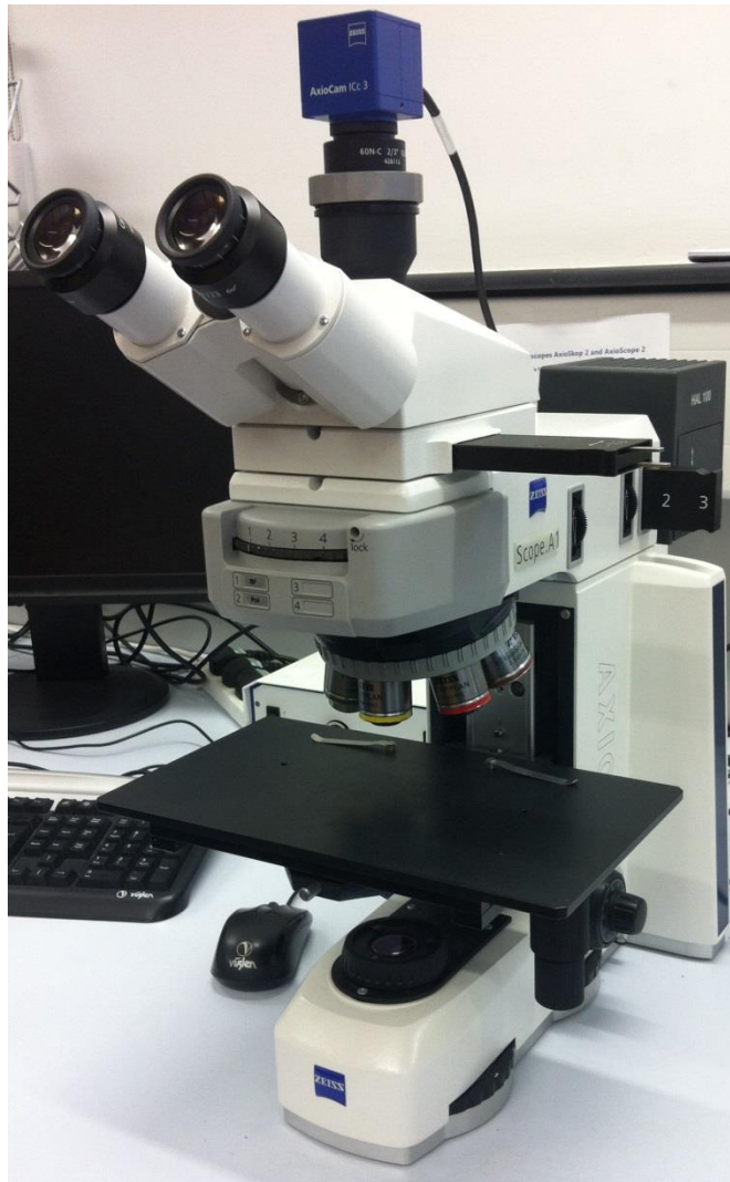
Figure 3.6 Microscope Axio Scope.A1 and its features
