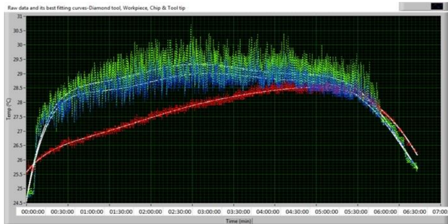
Figure 6.5 The best fitting curves of temperature partitioned distribution of cutting AA6082-T6 on diamond tool (blue dash line), workpiece (red dash line), and tool tip (green dash line) for whole cutting time interval ( ^{\circ}\text{C} - min)
