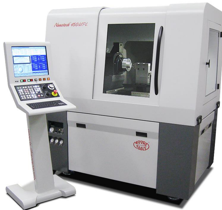
Figure 2.6 'Nanotech 450UPL' - Ultra-Precision 2-Axis CNC Diamond Turning Lathe produced by Moore Nanotechnology Systems, LLC
