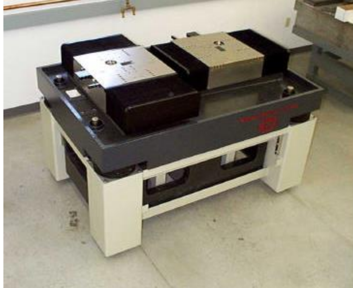
Figure 2.2 A current single point diamond turning machine with granite base and slides (Moore Nanotechnology Systems LLC)
