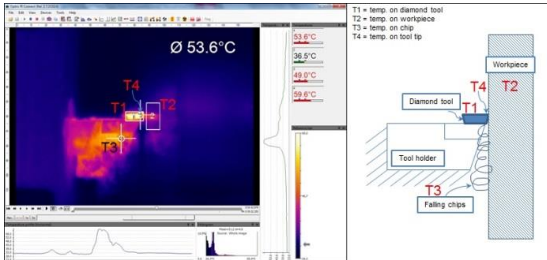
Figure 6.3 Cutting temperature and the associated heat partitioned distribution in micro cutting process
