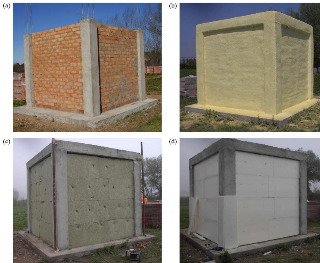
Figure 2.4 Test cubicles: (a) Reference cubicle; (b) cubicle insulated with PUR; (c) cubicle insulated with mineral wool; (d) cubicle insulated with polystyrene (Cabeza et al. , 2010)
