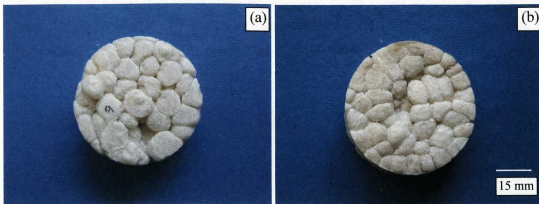
**Figure 8.8** The difference in appearance of the external surfaces at the top (a) and the bottom (b) for a Temple flour block.
