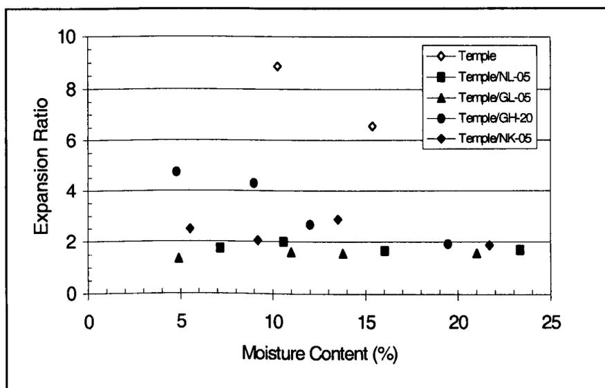
**Figure 6.3** Variation of expansion ratio with moisture content for the pellets extruded with different grades of PVA.
