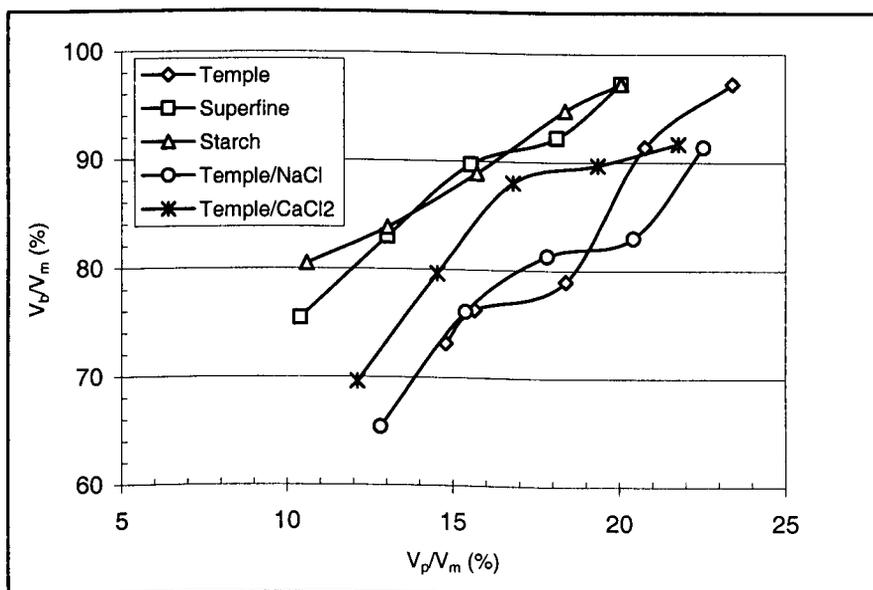
**Figure 8.6 Effect of initial loading of pellets on the final mould filling by foamed pellets.**
