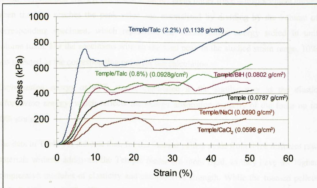
**Figure 7.8 Typical compressive stress – strain curves (22°C, 50% RH) for the microwave foamed pellets made from Temple flour and different additives.**
