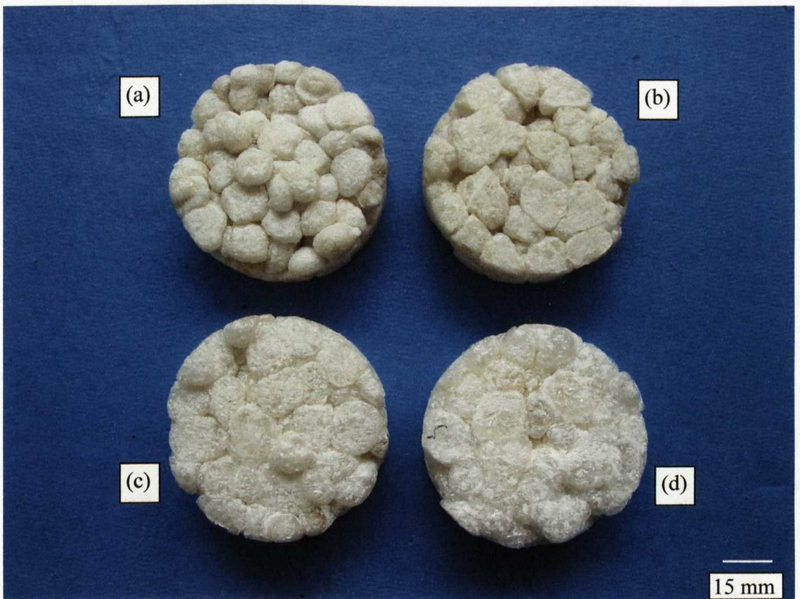
**Figure 8.9 Moulding surfaces showing difference in fusion for blocks made from (a) Temple flour; (b) Temple/ $\text{CaCl}_2$  (10.5%); (c) Superfine flour; (d) purified wheat starch.**
