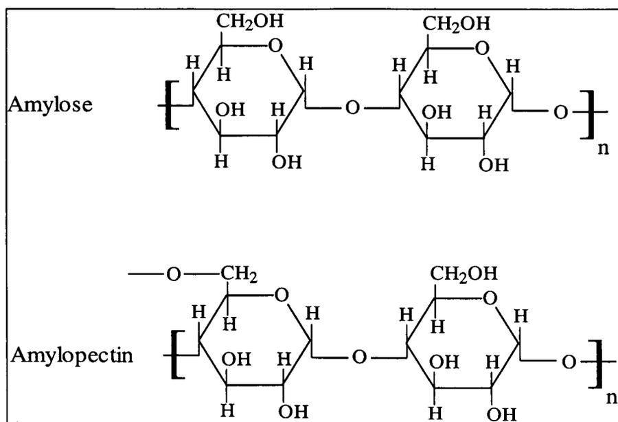
Figure 2.1 The schematic structure of amylose and amylopectin.
