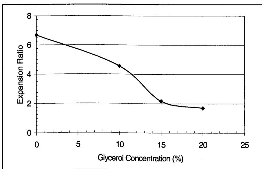
**Figure 6.9 Effect of glycerol concentration on the expansion ratio of extruded pure starch/glycerol pellets.**
