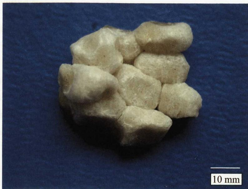
**Figure 8.2 Pellets showing faceted interfacial surfaces with good contacts in microwave foamed block.**
