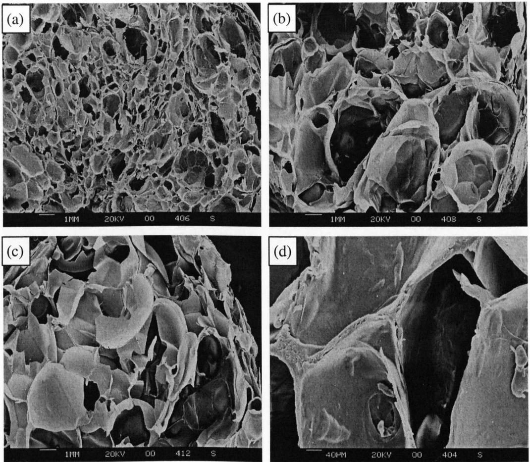
**Figure 7.4 Scanning electron micrographs of cross-sections of foamed pellets with different raw materials: (a) Temple flour, (b) Superfine flour, (c) Purified wheat starch, (d) cell wall in Temple foam shown in (a) at higher magnification.**
