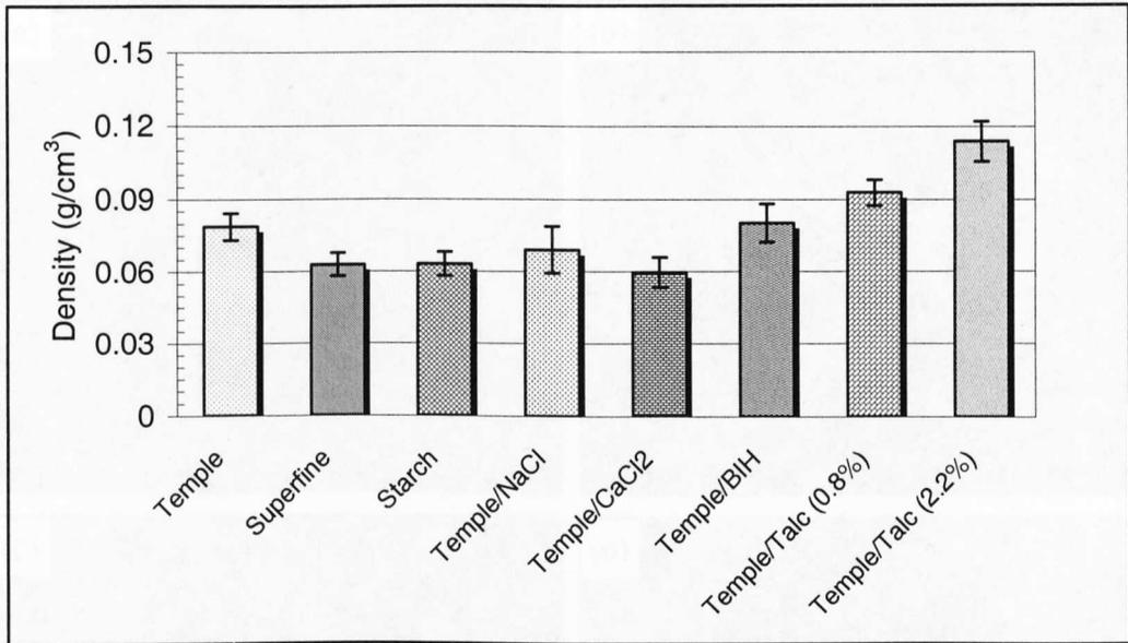
**Figure 7.3 Densities of microwave foamed pellets when the denser skin layer is removed.**
