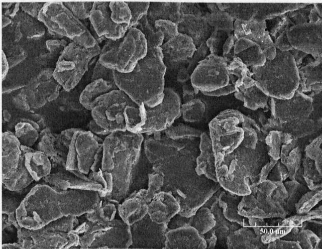
Figure 3.2 SEM micrograph of the particles in the talc powder.
