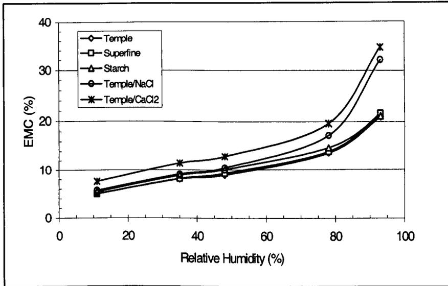
**Figure 7.6 Water absorption isotherms for the microwave foamed pellets with different compositions at room temperature.**
