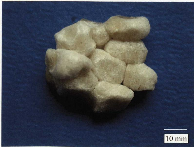
**Figure 8.2 Pellets showing faceted interfacial surfaces with good contacts in microwave foamed block.**
