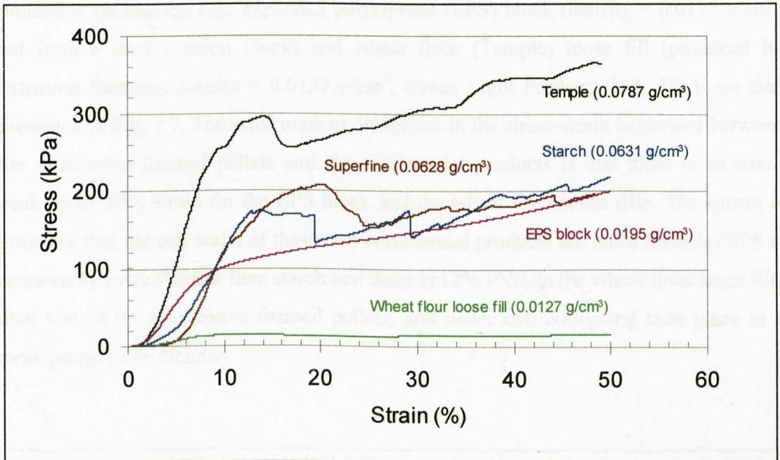
**Figure 7.7 Comparison of typical compressive stress–strain curves (22°C, 50% RH) for the microwave foamed pellets made from different raw materials with commercial protective packaging materials.**
