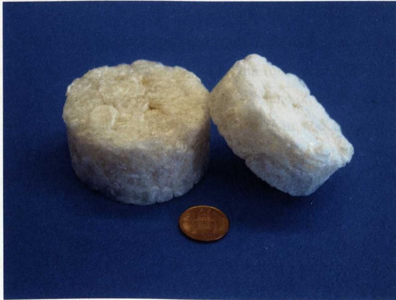
**Figure 8.5 Uniformly foamed starch based blocks using microwave heating.**
