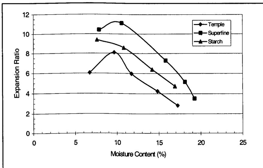
**Figure 5.9 Relationship between the expansion ratio and moisture content in the pellets extruded at same condition but with different raw materials.**
