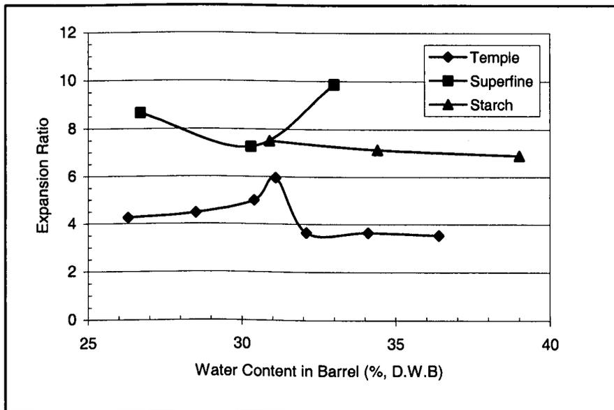
**Figure 5.8 Changes of expansion ratios with water content in barrel for the pellets extruded at 120°C with different raw materials.**
