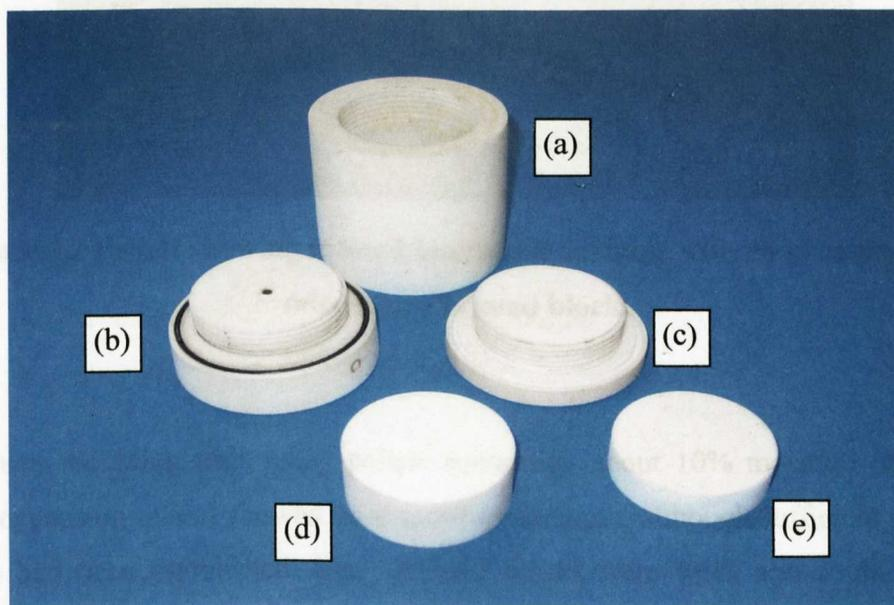
**Figure 8.1** PTFE mould used in this work. (a) the central cylindrical tubular mould; (b) & (c) the end caps; (d) & (e) discs for height adjustment of blocks.
