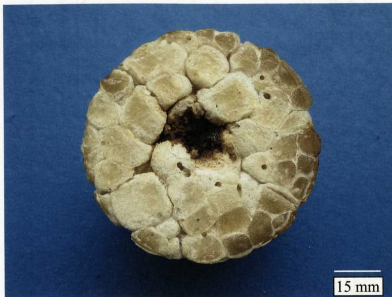
**Figure 8.3 A non-uniform foamed block with burnt centre and insufficiently foamed surface.**
