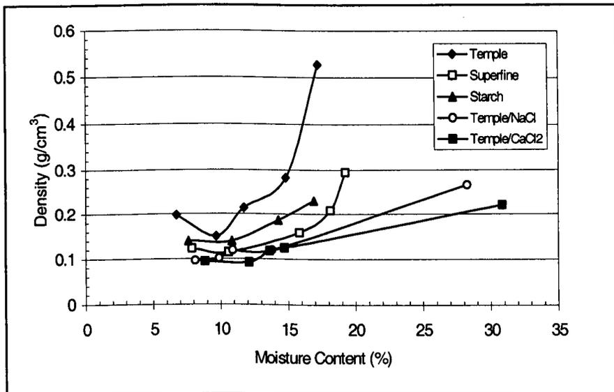
Figure 7.1 The densities of expanded pellets microwave foamed at different moisture contents.
