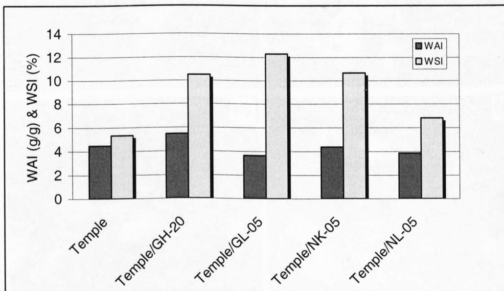
**Figure 6.6 WAI and WSI values for the pellets extruded with different grades of PVA.**
