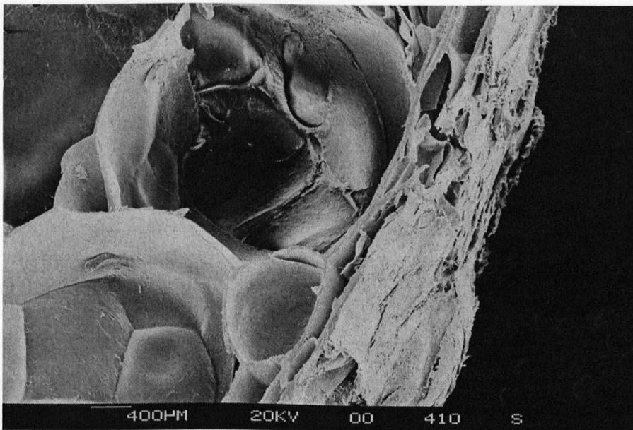
**Figure 7.2** The denser skin layer of microwave foamed the Superfine flour extruded pellet.
