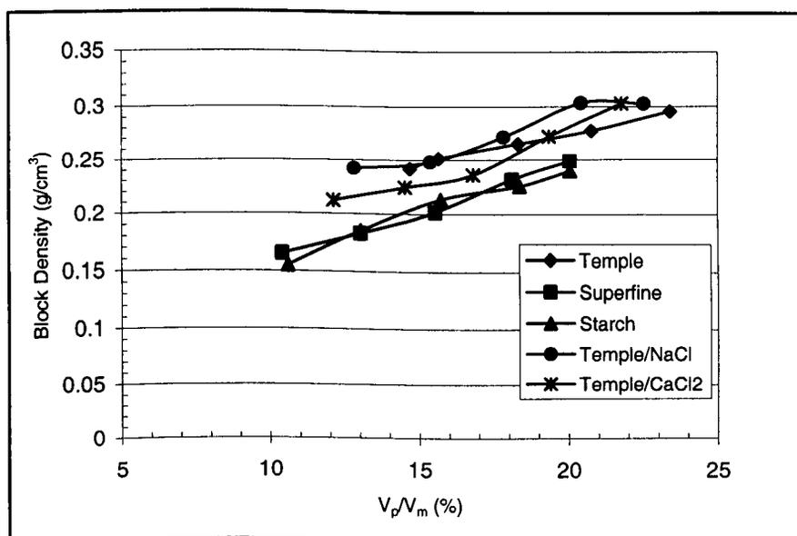
**Figure 8.7 Changes of foamed block density with initial loading of pellets of various compositions.**
