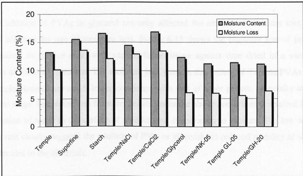
**Figure 6.12** Moisture content before microwave heating and moisture loss during microwave foaming of extruded pellets with different formulations.
