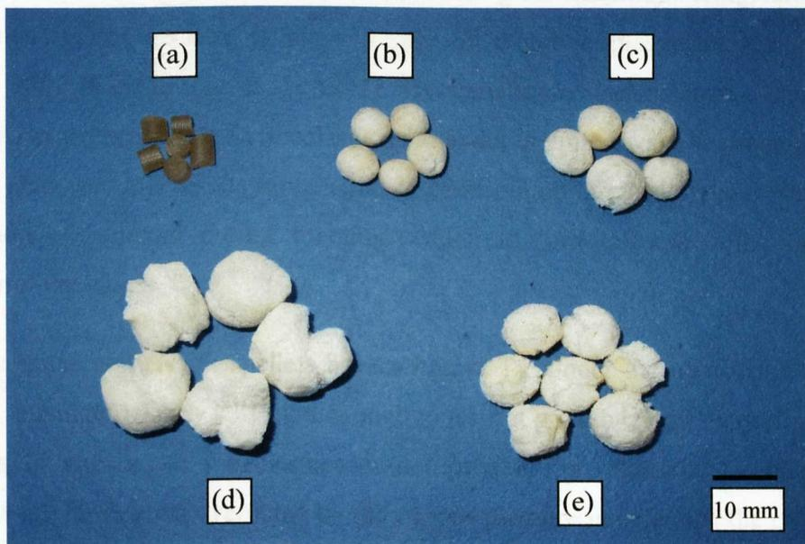
**Figure 5.6 Extruded Temple pellets microwave foamed at various moisture contents. (a) extruded pellets; (b) 17.2%; (c) 14.8%; (d) 9.7%; (e) 6.7%.**
