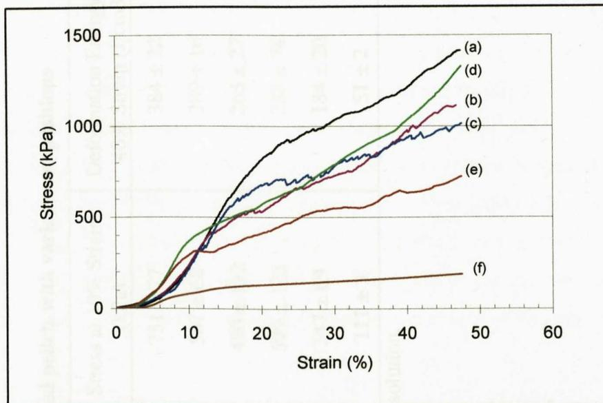
**Figure 8.11 Typical compressive stress - strain curves for the foamed blocks made from pellets with different compositions and density: (a) Temple flour ( $0.254 \text{ g/cm}^3$ ); (b) Superfine flour ( $0.215 \text{ g/cm}^3$ ); (c) Purified wheat starch ( $0.217 \text{ g/cm}^3$ ); (d) Temple/NaCl ( $0.226 \text{ g/cm}^3$ ); (e) Temple/ $\text{CaCl}_2$  ( $0.221 \text{ g/cm}^3$ ); (f) EPS block ( $0.018 \text{ g/cm}^3$ ).**
