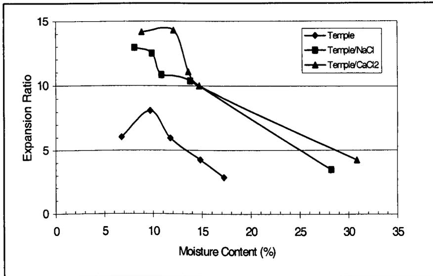
**Figure 6.11** Expansion ratio of extruded Temple flour with and without salts at different moisture content.
