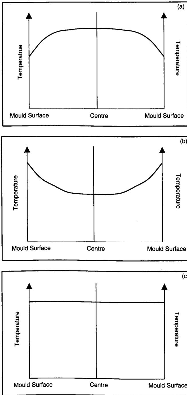
**Figure 8.4 Schematic diagrams showing likely temperature distribution with a moulding. (a) Microwave heating in a cold mould, (b) conduction heating in a mould, (c) combined heating of microwave in a preheated mould.**
