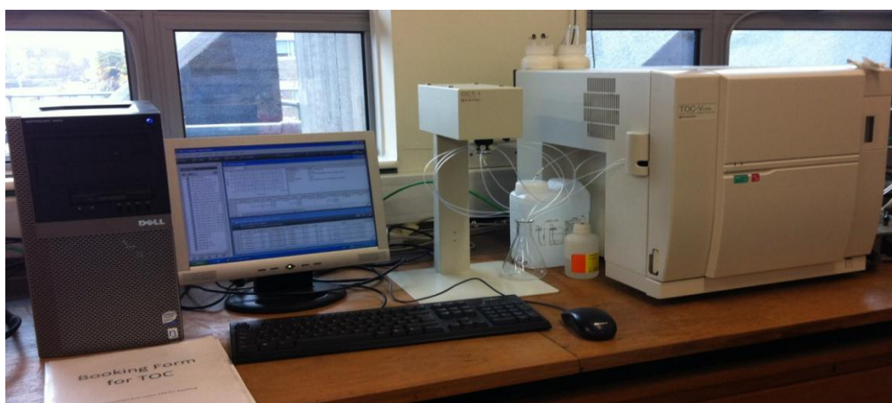
Figure 3.10: Total organic carbon analyser.
