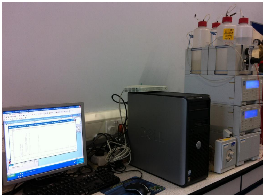
Figure 3.20: Ion chromatography system.
