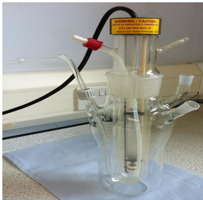
Figure 3.5: Assembled photolytic system.
