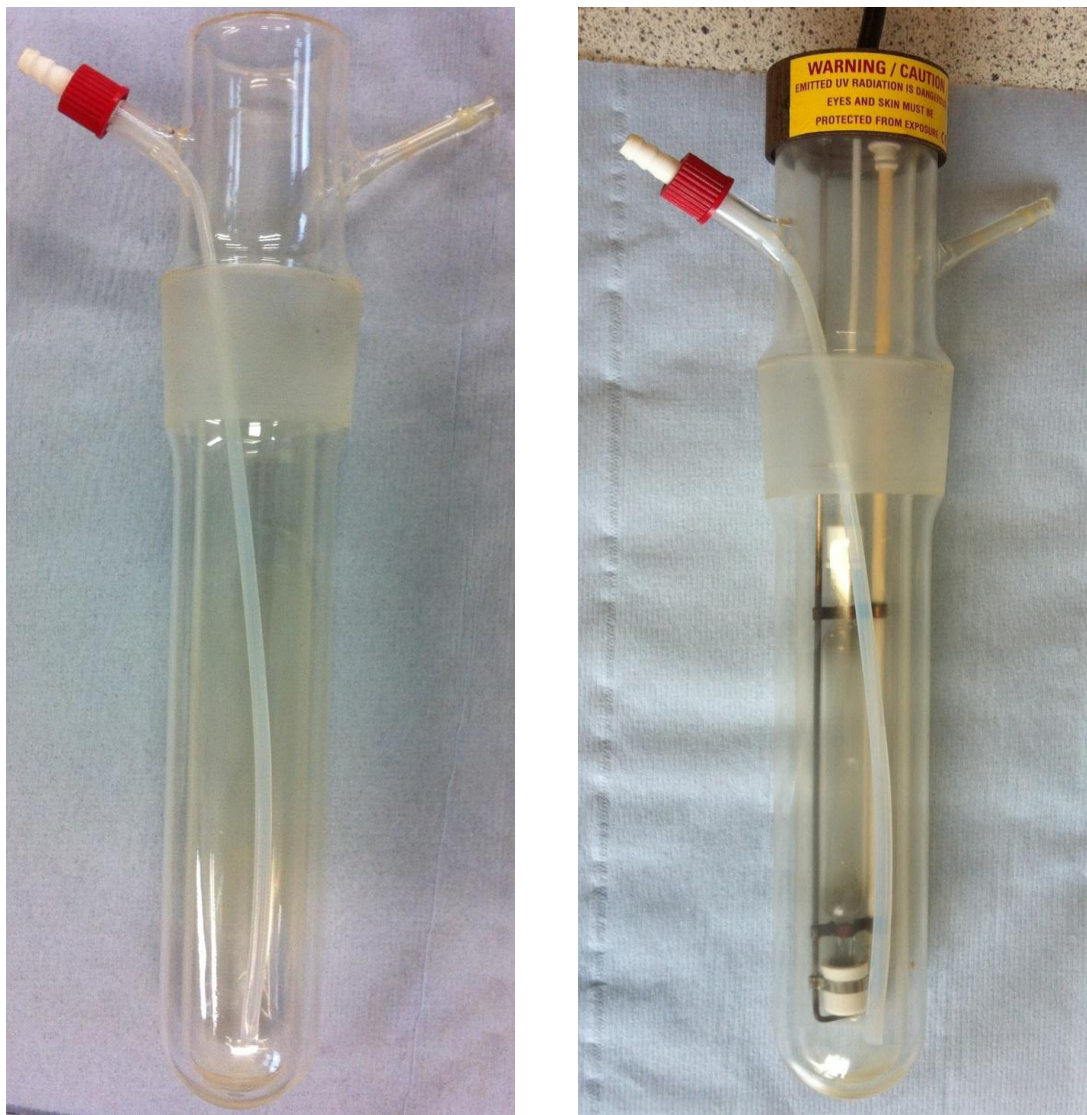
Figure 3.3: Two immersion wells – with and without the UV lamp.
