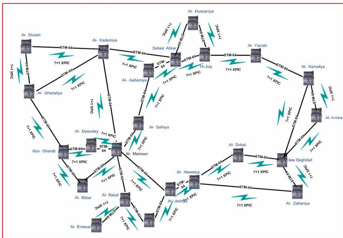
Figure 3.13: Network Overview 31 MW links, 31 Optical STM-64 links and 23 OMS
