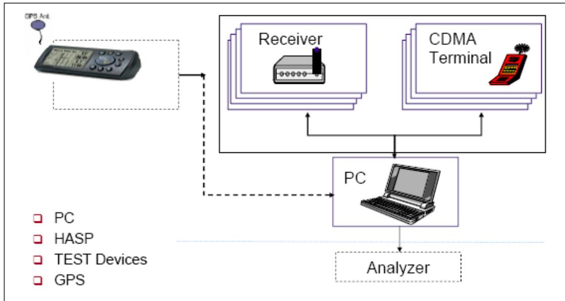
Figure 1-2: Drive test system configuration
