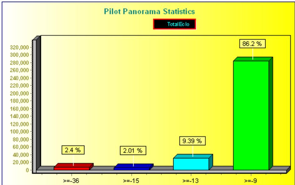
For the network, Ec/Io >= -9 is 86.2% and Ec/Io >= -13 is 9.39% of the tested areas. This also good ratio for normal communication.
