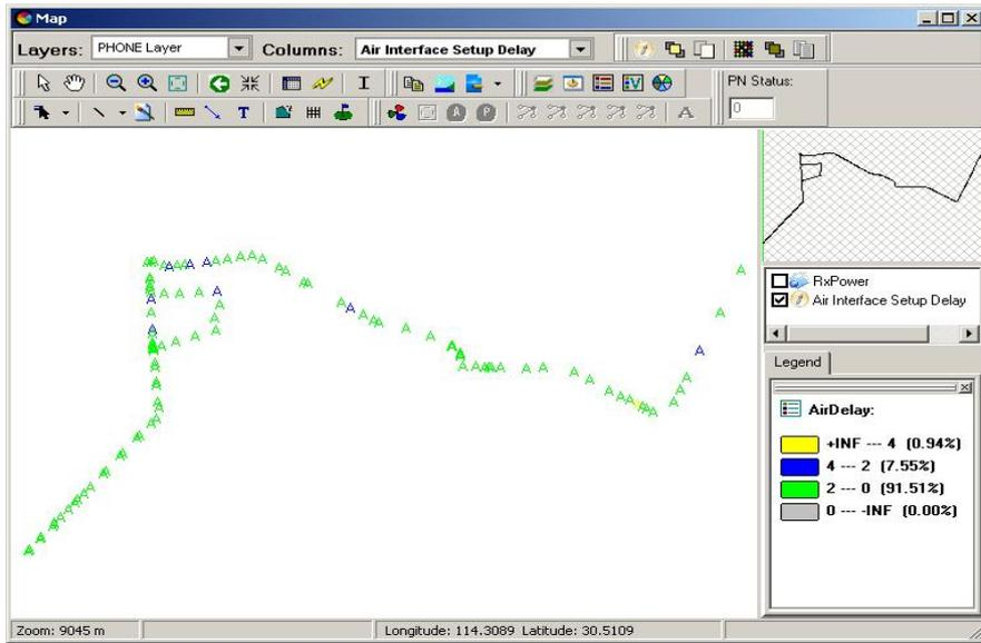
**Figure 6: Air interface Setup Delay geographic display**
