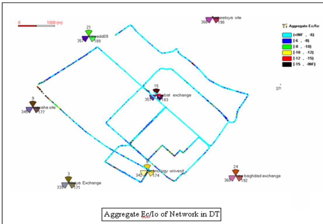
Figure 4.18: Aggregate Ec/Io DT measurements
