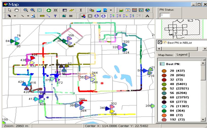
Figure 10: Pilot analysis – Strongest Ec/Io( Energy to Interference) analysis
