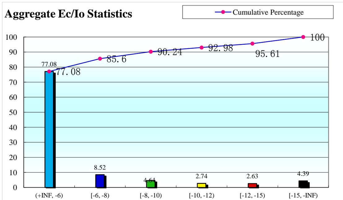
Figure 4.6: Aggregate Ec/Io Distribution
