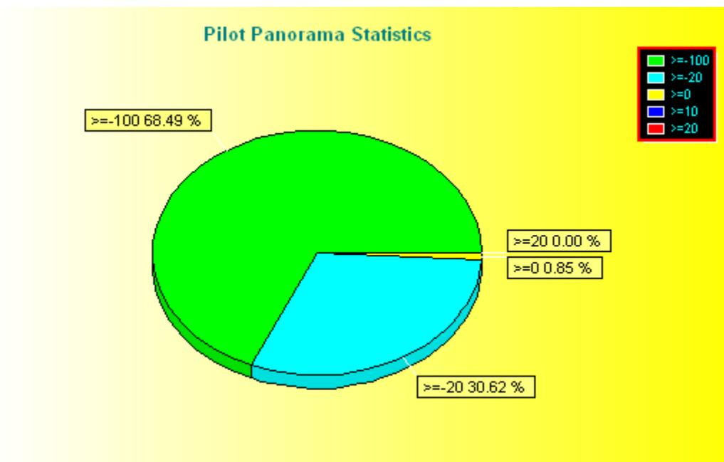
The Tx is good. That is the MS in 99.11 % of the tested area transmit power less than -20dBm.
