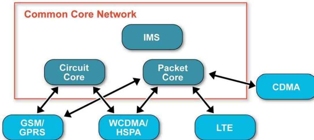
Figure 3.16: The common core network will enable roaming between GSM/EDGE, WCDMA/HSPA, LTE and CDMA.
