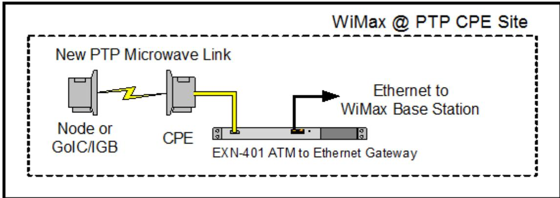
Figure 2.13: WiMax Interconnect using PTP Microwave
