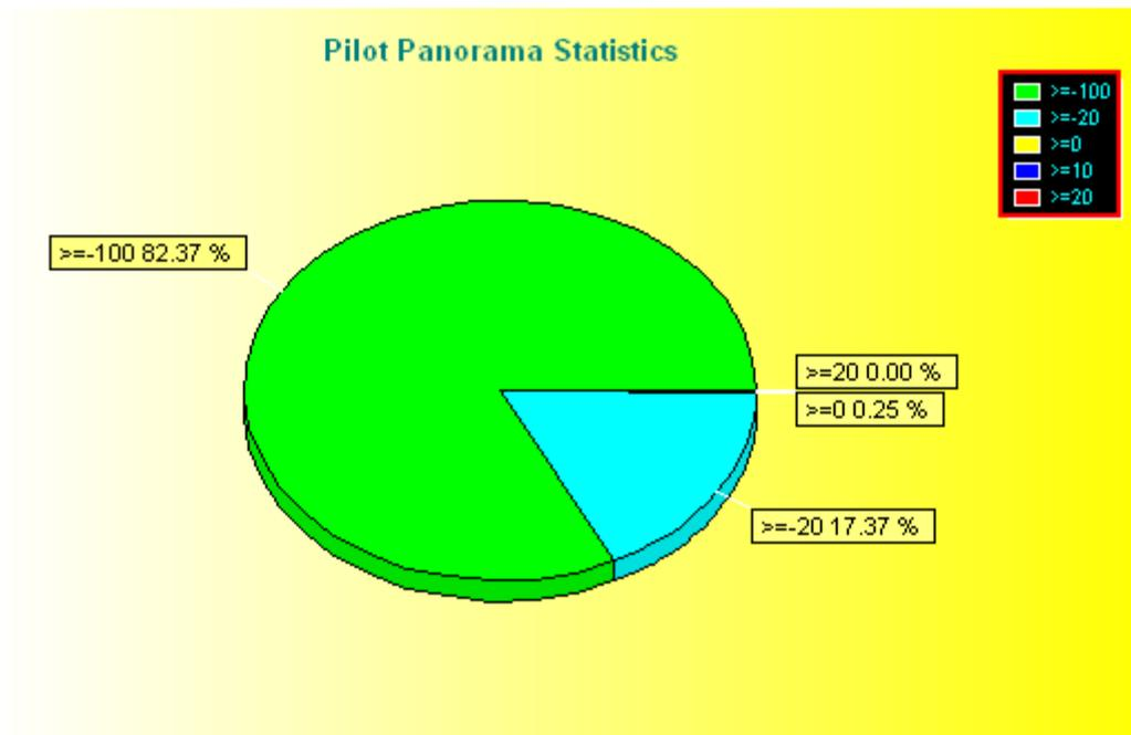
The Tx is good. That is the MS in 99.74% of the tested area transmit power less than -20dBm.
