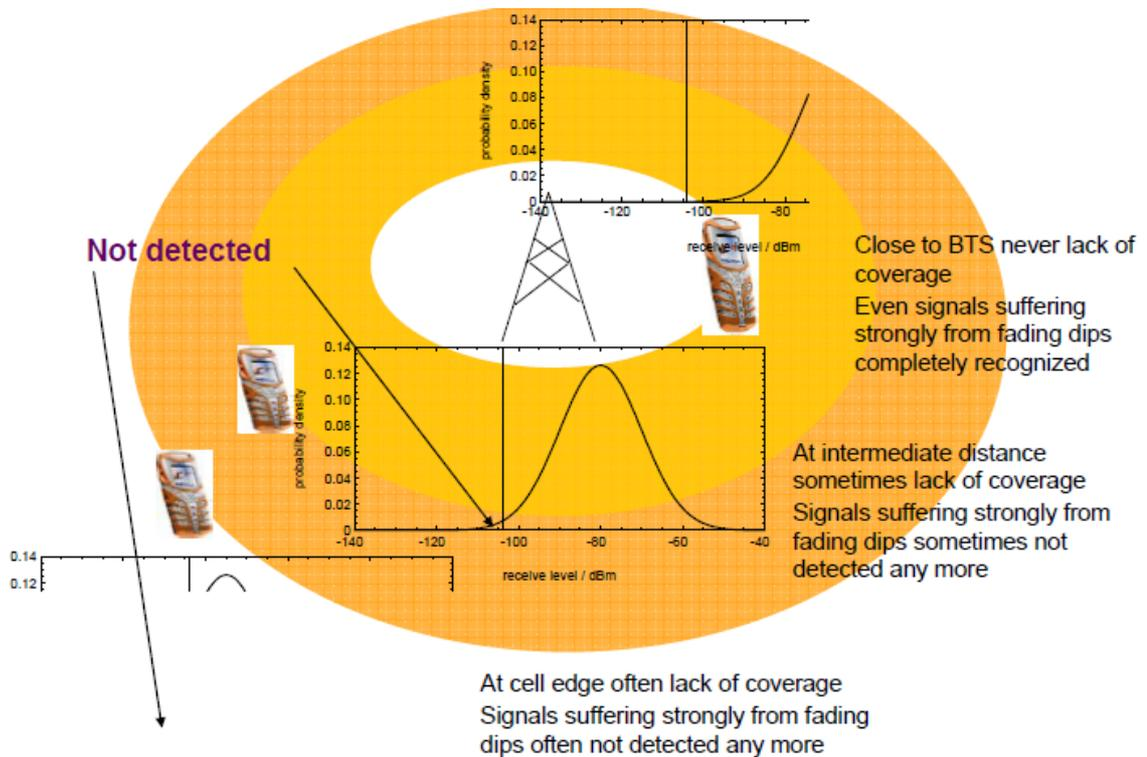
Figure 6.4: Coverage measurement signals strength
