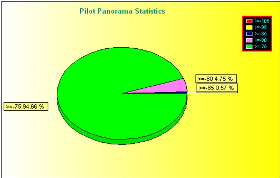
The areas that have very good Rx level (Rx  $\geq$  -75 dBm) are 94.66% of the total tested areas. Totally there are 99.41% of the total tested area have good Rx level (Rx  $\geq$  -80 dBm). This is a good ratio for indoor coverage.
