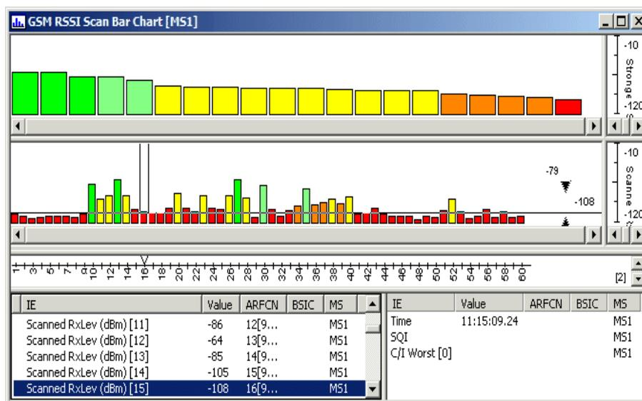
**Figure 126: Signal Strength Measurements**
