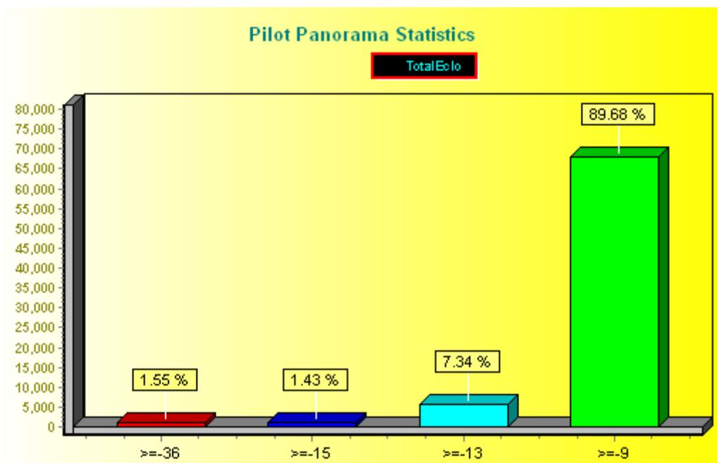
For the network,  $Ec/Io \geq -9$  is 89.68% and  $Ec/Io \geq -13$  is 7.34% of the tested areas.
