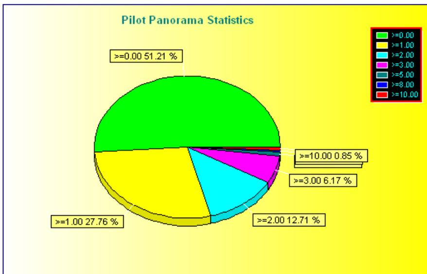
The areas that have FFER less than 3 are 91.68% of the total tested area. This is good ratio for voice service.
