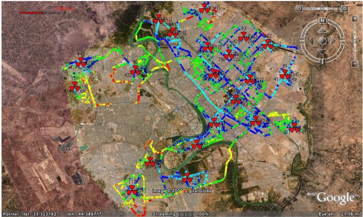
**Figure 4.3: Forward Received Power of Network in DT**
