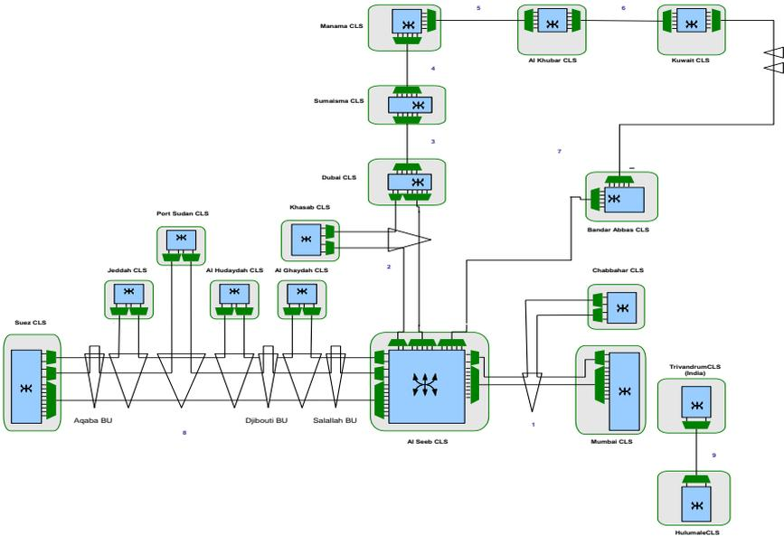
Figure 3.4: schematic configuration of the FALCON Network
