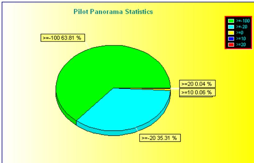
The Tx is good. That is the MS in 99.12% of the tested area transmit power less than -20dBm.
