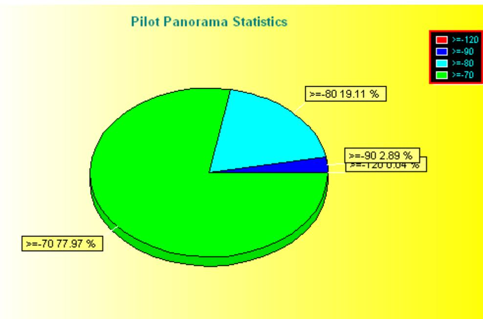
The areas of good Rx level are 77.97 & 19.11% so totally are 97.08 % of the total tested area. This is good ratio.
