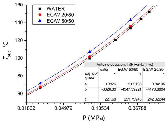
**Fig. 4.** Bubble point/Saturation temperature curves under different pressures.
