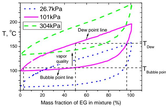
**Fig. 3.** Phase equilibrium diagram of ethylene glycol–water mixtures at different pressures.
