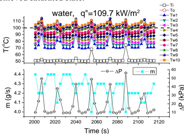
**Fig. 6.** Periodic instability of subcooled boiling in mini-tube.
