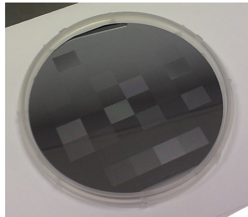
Figure 3 – Photograph of the silicon micro-structured surface produced at the SMC. The regions of different hue indicate different microstructure properties.
