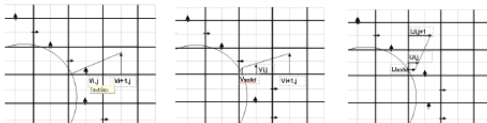
Figure 4: linear interpolation method: interpolating V_j for a stationary solid in vertical direction (left), interpolating V_j for a moving solid ( V_{solid} ) in vertical direction (middle); interpolating U_i for a moving solid ( U_{solid} ) in horizontal direction.
