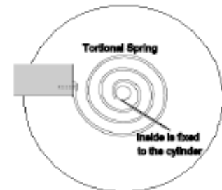
Figure 1 : Cylinder with Rotational degree of freedom, a Torsional spring- stiffness of K and the moment of Inersial of I
