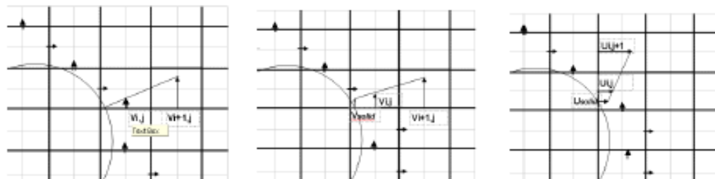
Figure 4: linear interpolation method: interpolating V_j for a stationary solid in vertical direction (left), interpolating V_j for a moving solid ( V_{solid} ) in vertical direction (middle); interpolating U_{ij} for a moving solid ( U_{solid} ) in horizontal direction.
